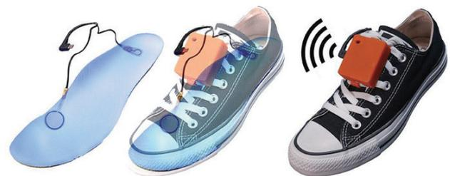
**Fig. 2.** Electroskip sensor positioning under toes and heel.
