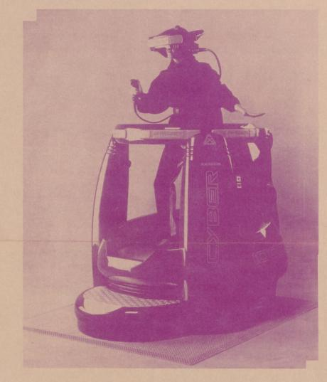
dimensional scene. The scene is altered according to every movement of the person wearing VISETTE headgear, thereby creating for the player the illusion of being totally immersed in the visual aspects of the game environment. A press of a thumb-button on the SPACESTICK moves the player forward and upwards in the "cyberspace", while a squeeze of a trigger launches a rocket grenade at an adversary, or at a pterodactyl, if it hasn't already snatched up its victim.
